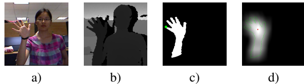
Fig. 1: Extraction of the hand samples: a) Acquired color image; b) Acquired depth map; c) Extracted hand samples (the closest sample is depicted in green); d) Output of the Gaussian filter applied on the mask corresponding to \mathcal{H} with the maximum (i.e., C_g ) in red; ( Best Viewed in colors ).
